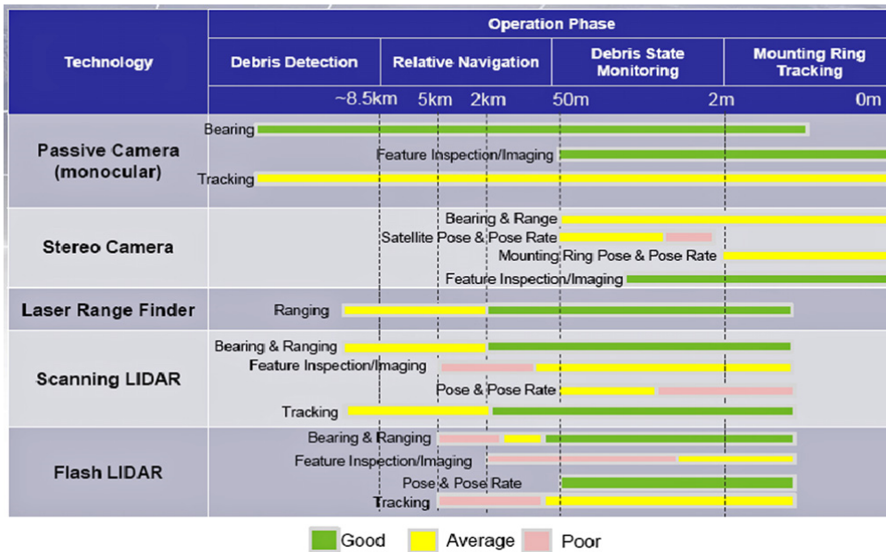
Figure 10 Typical technologies usable for short-range rendezvous between Chaser and Debris Appendix H shows the status of significant approaching technologies.
