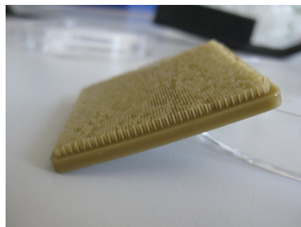
Figure 31 Gecko materials produced by the Leibniz Institute of New Materials
